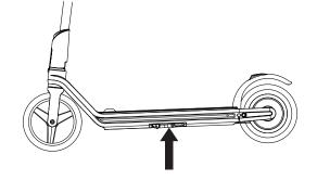
Step 3: Grip both hands on handle bar. Use one foot gently press on the accelerator pad. To accelerate, press accelerator pad downwards. To deccelerate, lift up from accelerator pad.
