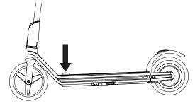
Step 4: To brake or stop, place other foot on the mud flap. Presss down on mud flap as needed to reduce speed or come to a complete stop.
