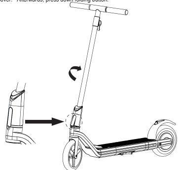
Step 2: Fold down stearing pole, press pole towards mud flap until Utility / Locking Hook until it is lock into place.
